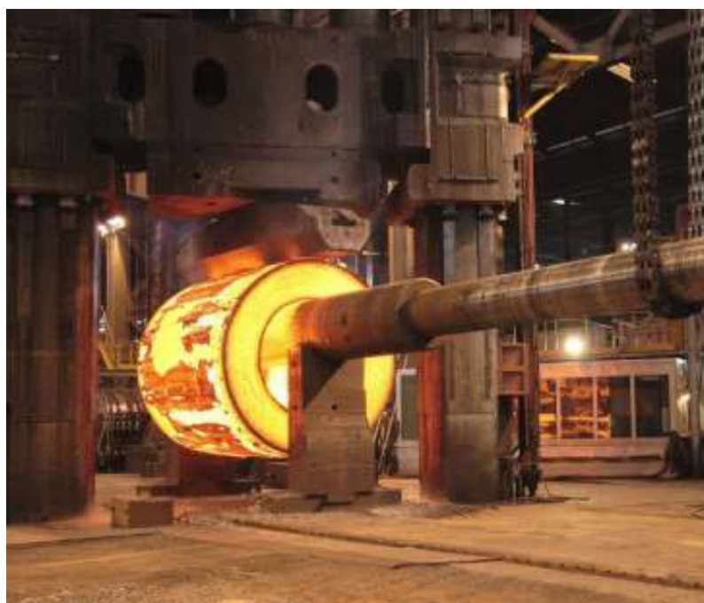
Hammer forging and descaling a reactor shell at SFAR Steel
