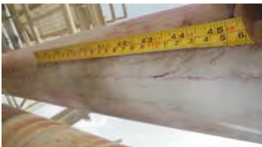
Fig. 6b: Linear Indication in Locations at the Burnery Side
