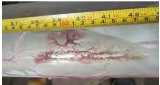
Fig. 6b: Linear Indication in Locations at the Burnery Side
