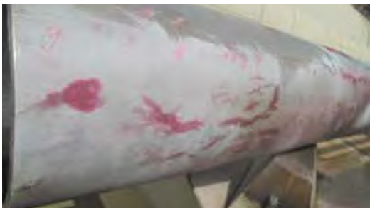
Fig. 6a: Linear Indication in Locations Close to the Rupture
