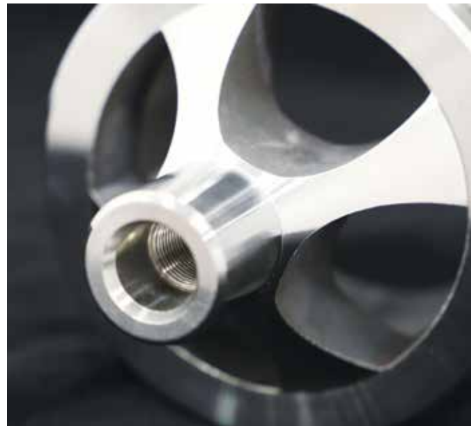
3D printed 316 stainless steel valve plug
