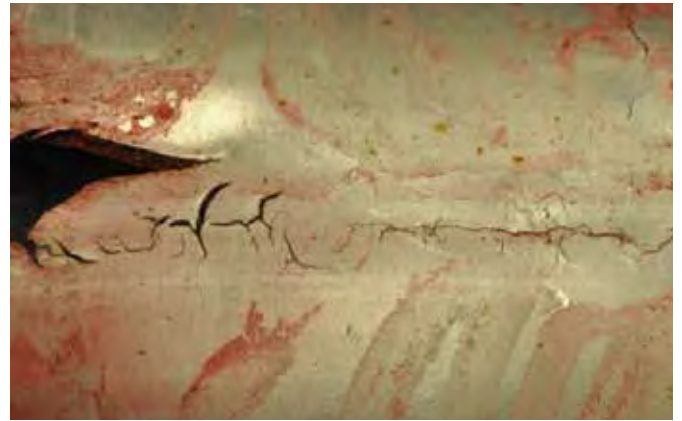
Fig. 1c: Cracks adjacent to the rupture
