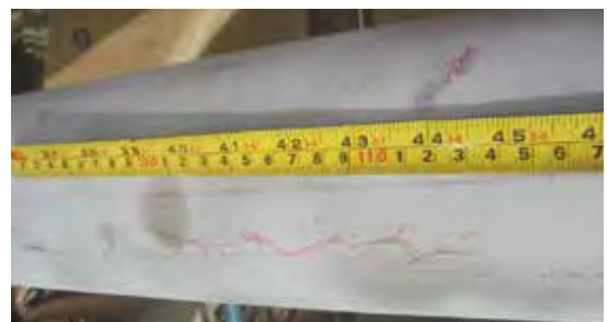
Fig. 6a: Linear Indication in Locations Close to the Rupture
