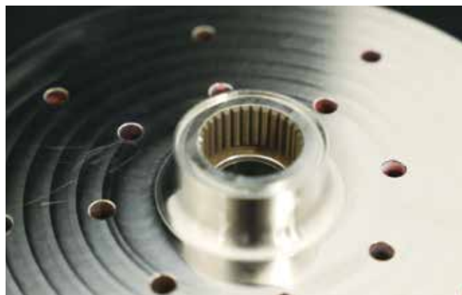
3D printed Titanium impeller
